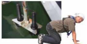
The transducer bracket prepared for shipboard testing. It would have been better to test both the analog echo sounder and the digital ones exactly at the same time and same location. However, we carried out tests by changing over switches of those echo sounders at a certain time interval to prevent interference between them.
